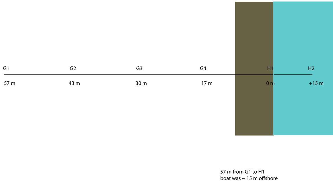
Figure 4: The schematic of the set-up at the Woodfibre LNG site. The brown coloration shows the dock and the blue indicates the water. Geophones are denoted as G1, G2, G3, and G4 and Hydrophones H1 and H2.
