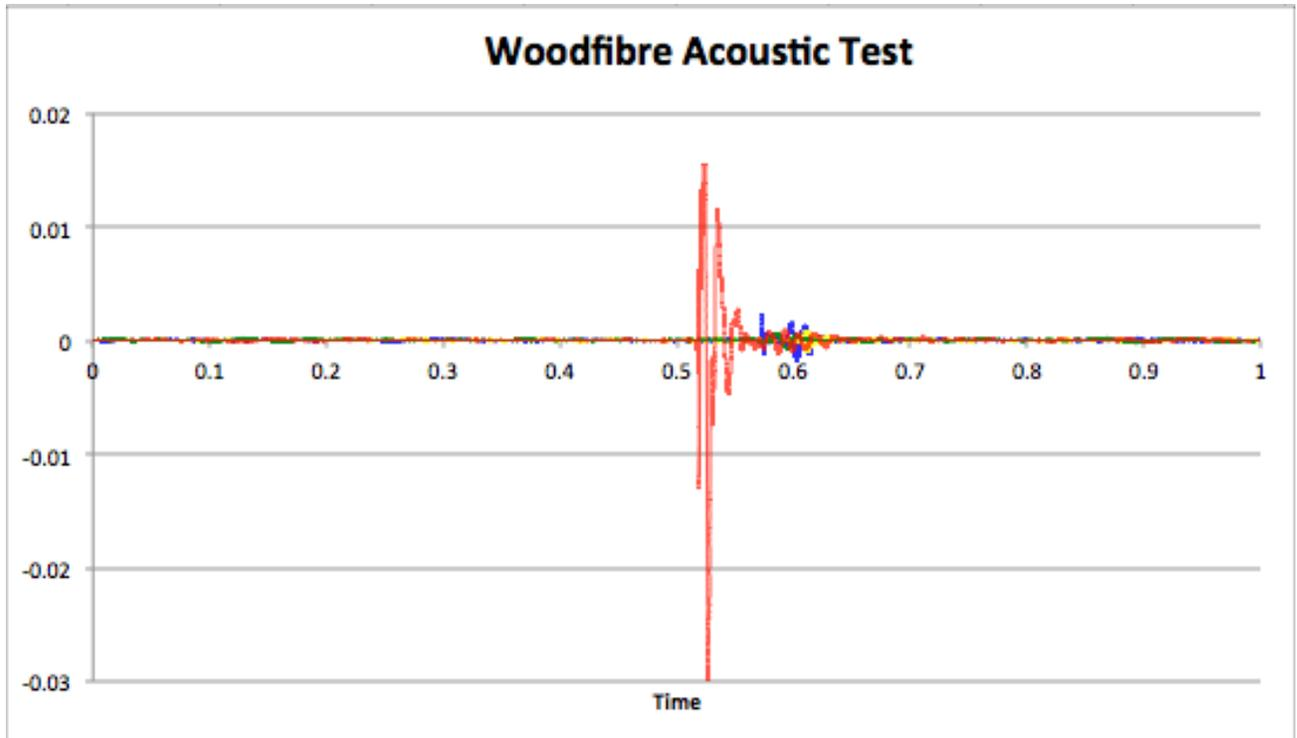
Figure 10: The signal as it passes through the Geophones at the Woodfibre site. We can see every signal at different amplitudes. G1 is denoted in blue, G2 in yellow, G3 in green, and G4 in red. The shot was initiated at G3.
