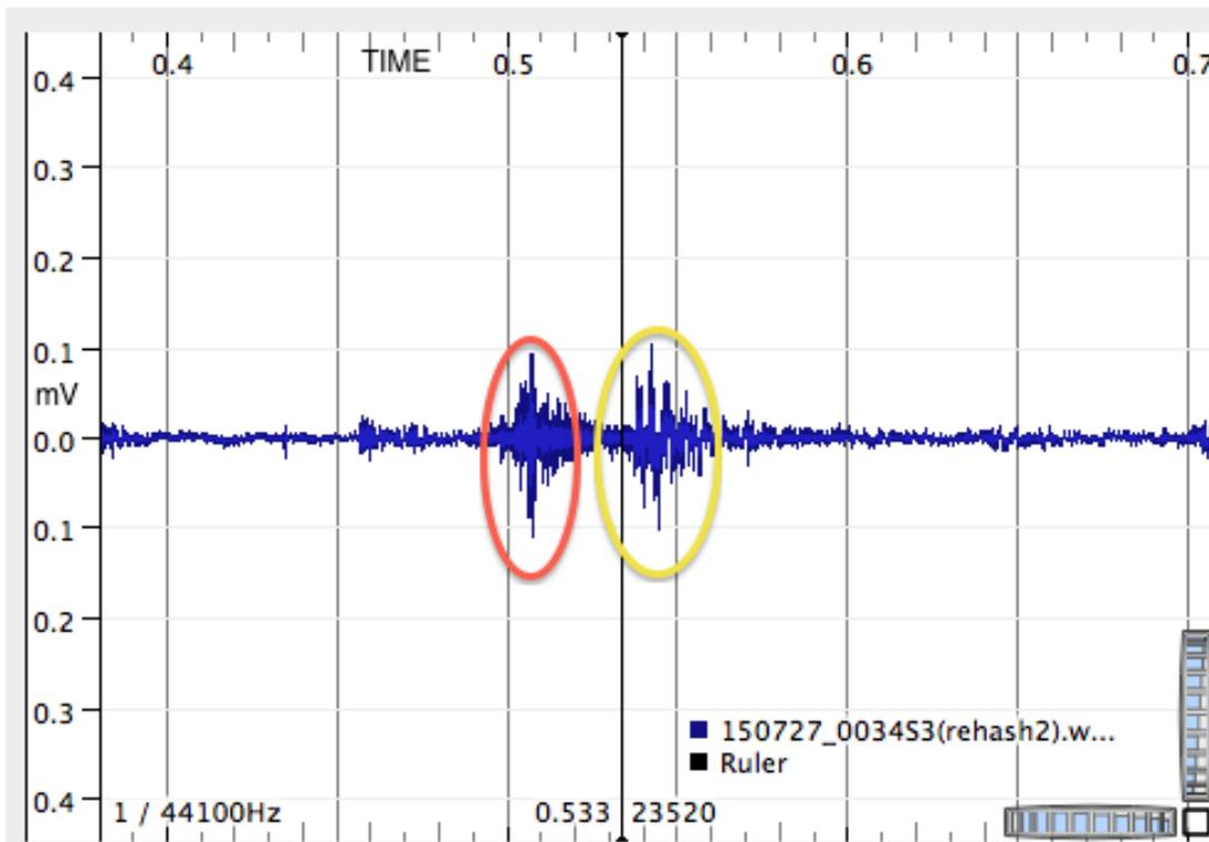
Figure 6: The signal as a waveform when it passes through H1 at a depth of 5m. We see the amplitude as mV (millivolts) on the Y-axis and time on the X-axis. The red oval is showing the initial signal and the yellow is showing it as it goes past. This image was modified from Sonic Visualizer.
