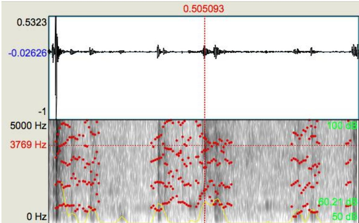
Figure 7: This image is showing a waveform of the signal as well as the spectrogram. Axes are showing Hertz (hz) and time. The grey background is the different frequencies, the darker the color the greater the frequency. The red dots are the formants, which is showing us the bands in the frequencies. The yellow line in the image is the waveform (figure 6). The decibels are shown as the green letters from 50dB to 100dB.
