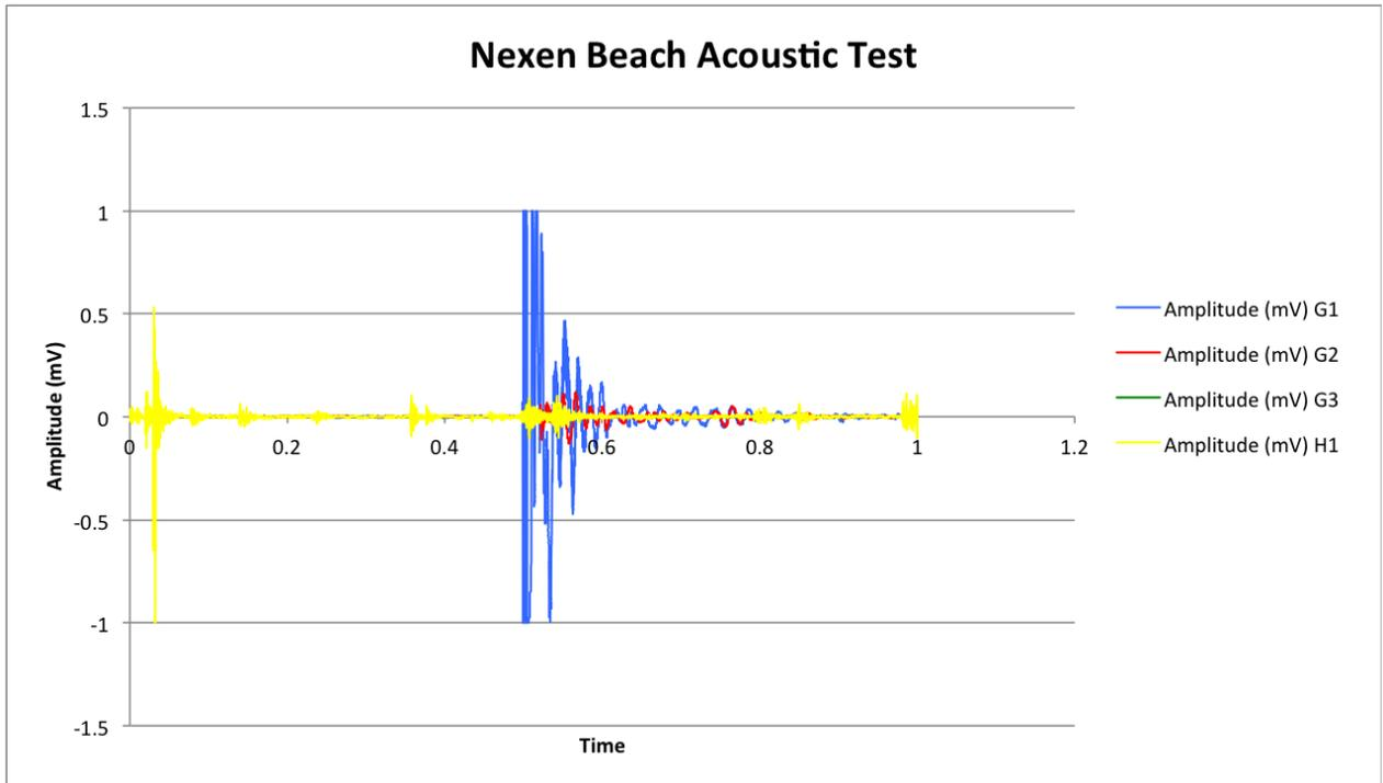
Figure 9: This graph shows us that the signal travels through the site, in all the sensors, and into the water where it has the possibility to cause issues. The data from G3 does not appear as the signal is too low.
