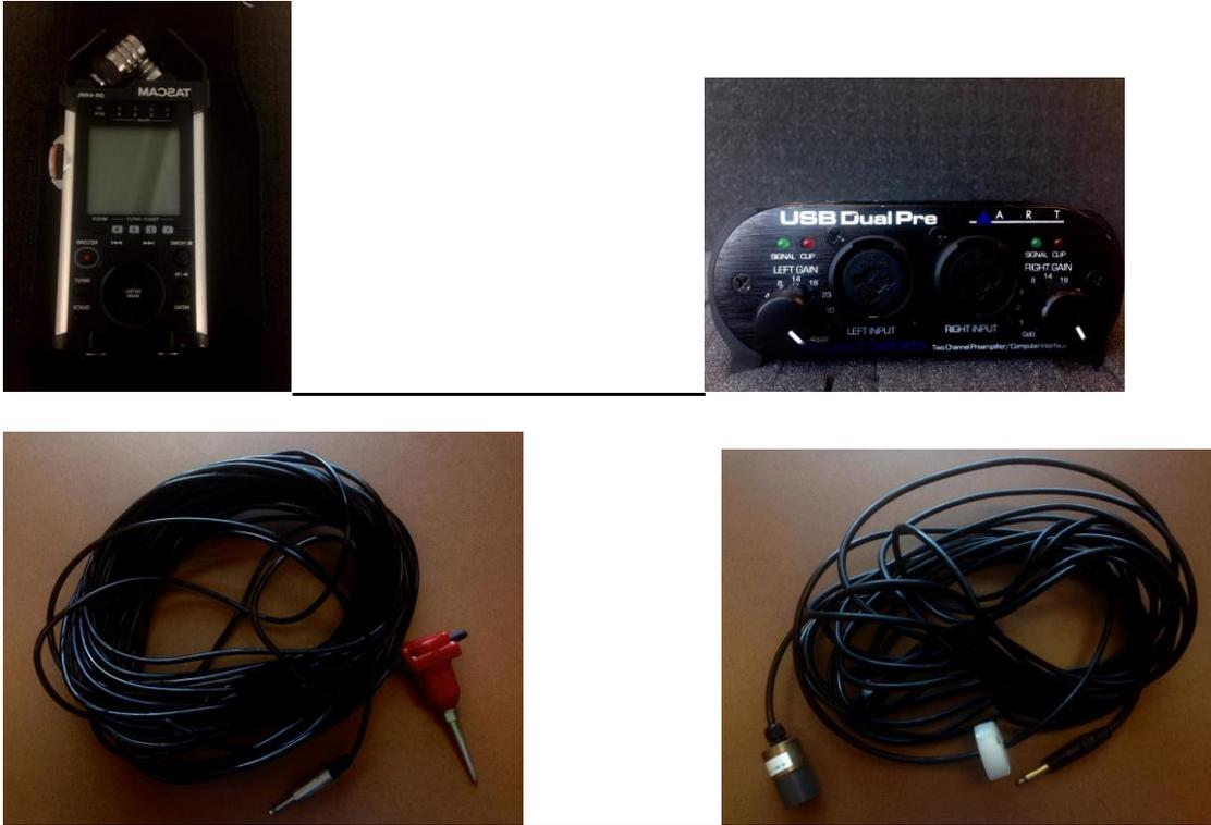
Figure 4. Equipment used in this study. Top left, TASCAM DR-44WL Recorder, top right, A.R.T USB Pre-Amplifier, bottom left RT Clark 4.5hz Geophone, and bottom right Cetacean Researchs CR1 Hvdrophone.
